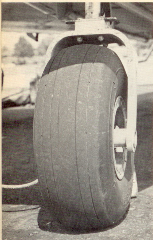
A tire with more than 80% tread wear, whether on your nose wheel or main gear, needs only a good dew to cause a total traction loss on a smooth paved runway.
